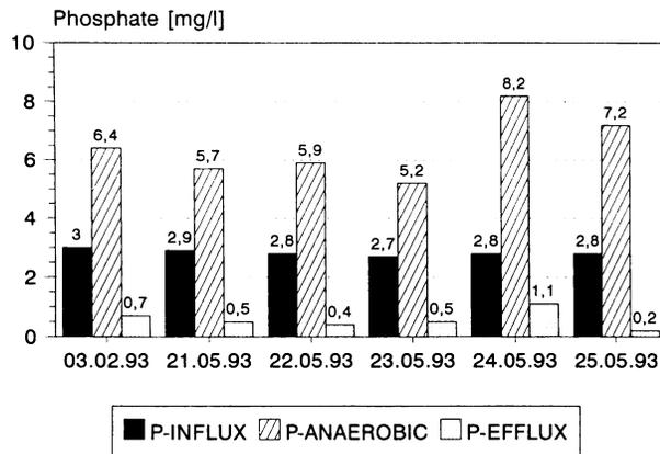
FIG. 5. On-line phosphate (P) determination in the Hirblingen plant for the sampling dates shown (day.month.year). The plant was in the EBPR mode without chemical phosphate precipitation on 3 February 1993 and in the EBPR and chemical phosphate precipitation mode on 21 May 1993. Acetic acid was added from 22 to 25 May 1993.
