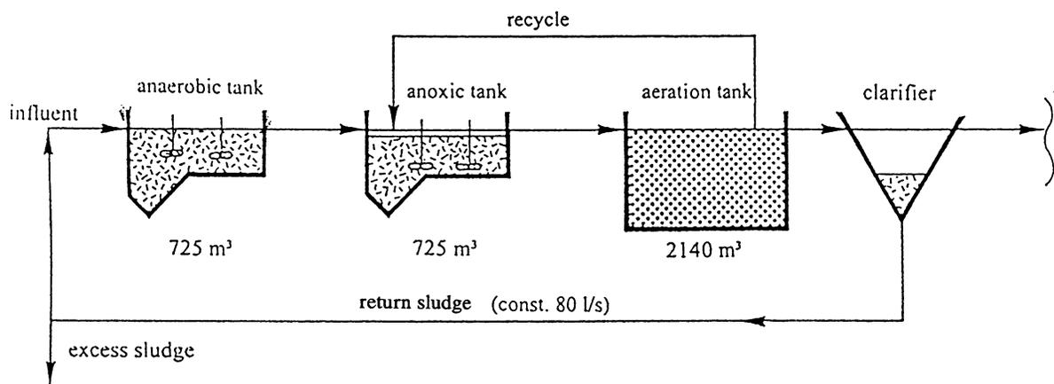
FIG. 1. Process schematic and reactor volumes of the Hirblingen, Germany, wastewater treatment plant.
